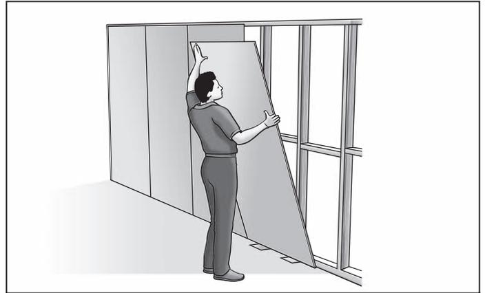
FIGURE 4 SHEET INSTALLATION
