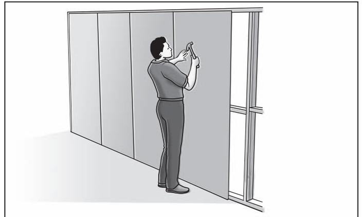
FIGURE 5 SHEET INSTALLATION
